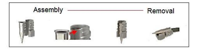
Image above shows a nozzle core assembled and removed from a reusable hub. Nozzle core flange is aligned with internal groove at top of hub and pushed through tapered vertical slot until seated.
