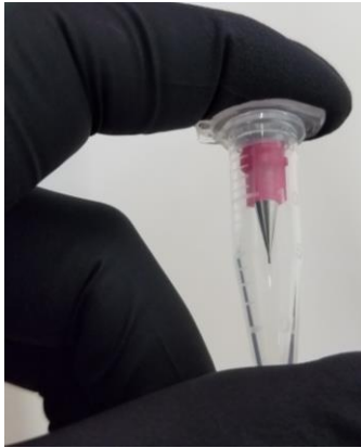
Image is a nozzle hub lodged inside lid of packing tube.
